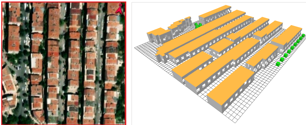
Figure 3.16. Satellite Image (left) and 3D Model (right) of the selected Urban Block 11 - İvedik
